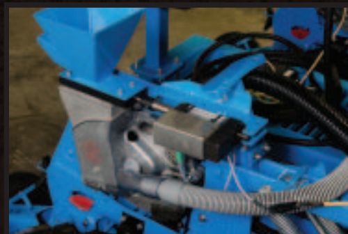
Electro-mechanical actuators control gates and valves.
